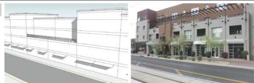
This articulation chart explains techniques for reducing the perceived mass of new construction in the Stockyards districts.
